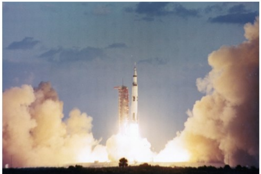
Saturn V launch – Smoke from flame trench is mostly Water System steam.
